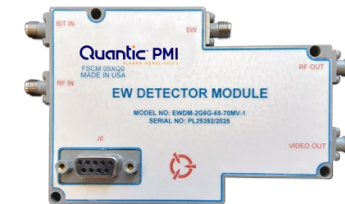
6 to 18 GHz, CW Immune, EW Detector Module
